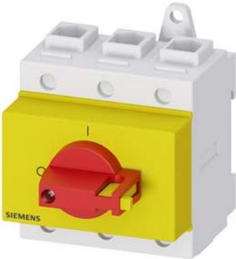
SENTRON, Switch disconnector 3LD, emergency switching-off switch, 3- pole, Iu: 125 A, operating power / at AC-23 A 400 V: 45 kW, installation in distribution boards, knob-operated mechanism, Red / yellow, handle direct at the switch
