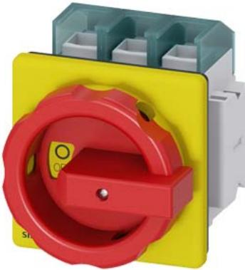
SENTRON, Switch disconnector 3LD, emergency switching-off switch, 3- pole, Iu: 125 A, operating power / at AC-23 A 400 V: 45 kW, front-mounted, 1 NC, 1 NO, rotary operating mechanism, Red / yellow, 4-hole mounting of the handle
