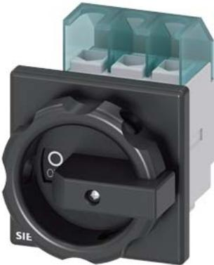
SENTRON, Switch disconnector 3LD, main switch, 3-pole, I<sub>u</sub>: 32 A, Operating power / at AC-23 A at 400 V: 11.5 kW, front-mounted, rotary operating mechanism, black, 4-hole mounting of the handle
