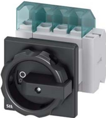
SENTRON, Switch disconnector 3LD, main switch, 4-pole, Iu: 25 A, Operating power / at AC-23 A at 400 V: 9.5 kW, front-mounted, 1 NC, 1 NO, rotary operating mechanism, black, Central mounting 22.5 mm of the handle
