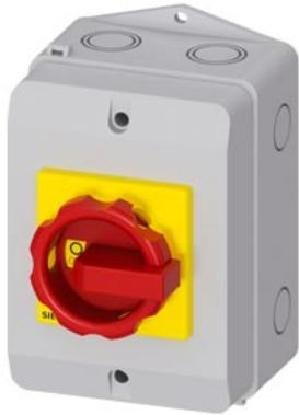
SENTRON, Switch disconnector 3LD, emergency switching-off switch, 3- pole, Iu: 16 A, operating power / at AC-23 A 400 V: 7.5 kW, Molded plastic encapsulation for inch cable gland, rotary operating mechanism, red/yellow
