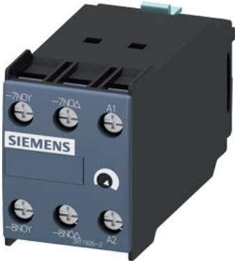
Solid-state time-delayed auxiliary switch, can be snapped on at the front, time range 1.5...30s, 200 ... 240 V AC, 2 NO, star-delta (wye-delta) function, sizes S6...S12
