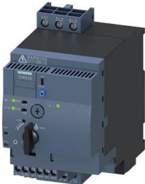
SIRIUS Compact load feeder Reversing starter 690 V 24 V AC/DC 50...60 Hz 0.32...1.25 A IP20 Connection main circuit: Screw terminal Connection control circuit: screw terminal
