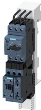
Fuseless motor starter Direct start 600VAC Size S0 1.8-2.5A 110/120VAC 50/60HZ screw connection For snapping onto 60 mm busbar systems Type of coordination 2 IQ = 150 KA Also full fills type Of coordination 1 1NO+1NC (contactor)
