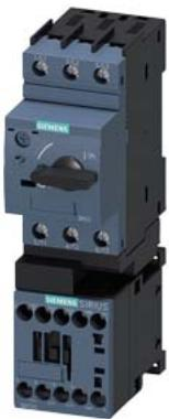
Fuseless motor starter Direct start 600VAC Size S00 0.45-0.63A 220/240VAC 50/60HZ screw connection For screw mounting Or 35 mm rail-mounting Type of coordination 2 IQ = 150 KA Also full fills type Of coordination 1 1NO (contactor)
