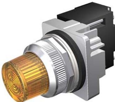
30mm Command/52, Chrome Finish Heavy Duty, Watertight/Oiltight Complete Metal Unit Illuminated Indicator Light Transformer type, 480V AC Super Bright LED Lamp, BA9s Glass Lens, Amber UL Listed, CSA Certified NEMA 1,3,3R,4,4X,12,13 & Automotive Standards
