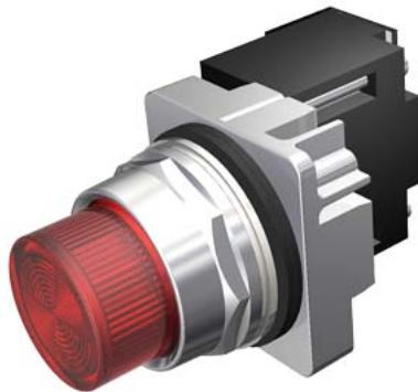
30mm Command/52, Chrome Finish Heavy Duty, Watertight/Oiltight Complete Metal Unit Illuminated Indicator Light Transformer type, 120V AC LED Lamp, BA9s Plastic Lens, Red UL Listed, CSA Certified NEMA 1,3,3R,4,4X,12,13 & Automotive Standards
