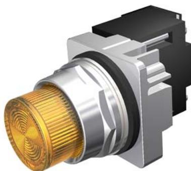
30mm Command/52, Chrome Finish Heavy Duty, Watertight/Oiltight Complete Metal Unit Illuminated Indicator Light Full Voltage type, 6V AC/DC LED Lamp, BA9s Plastic Lens, Amber UL Listed, CSA Certified NEMA 1,3,3R,4,4X,12,13 & Automotive Standards
