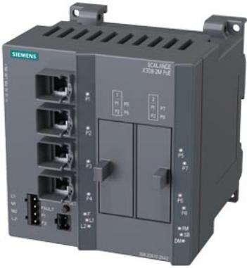
SCALANCE X308-2M PoE; managed IE switch, compact; 4x 10/100/1000 Mbit/s for RJ45 ports electrical with PoE; 2x 100/1000 Mbit/s for 2-port media modules, electrical or optical; LED diagnostics, error signaling Contact with select/set pushbutton, PROFINET IO device, network management, Integrated redundancy manager, office features (RSTP, VLAN, IGMP,..) C-plug in scope of supply.
