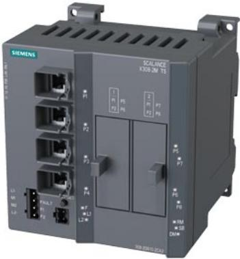
SCALANCE X308-2M TS; managed IE switch, compact; 4x 10/100/1000 Mbit/s for RJ45 ports electrical; 2x 100/1000 Mbit/s for 2-port media modules, electrical or optical; LED diagnostics; error signaling Contact; PROFINET IO device; network management; integrated redundancy manager; Office features (RSTP, VLAN, IGMP...); C-plug in scope of delivery extended temperature range with railway approval EN 50155;
