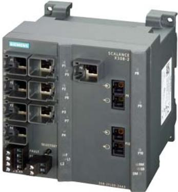
SCALANCE X308-2, managed plus IE switch, 2x 1000 Mbit/s MM SC 1x 10/100/1000 Mbit/s and 7x 10/100 Mbit/s RJ45 ports, LED diagnostics, error signalling contact with select/set pushbutton, PROFINET IO device, network management, integrated redundancy manager, office features (RSTP, VLAN, IGMP,...) C-PLUG in scope of supply.
