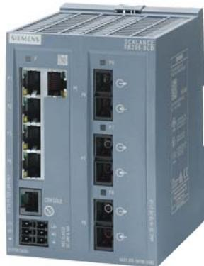
SCALANCE XB205-3LD managed layer 2 IE switch 5x 10/100 Mbit/s RJ45 ports 3x SM FO SC-port 1x console port, diagnostics LED redundant power supply; IEC 62443-4-2 certified; temperature range 0 °C to +60 °C; DIN-rail mounting; default EtherNet/IP.
