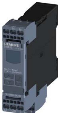
!!! product phase-out !!! the preferred successor is 3UG5842-2AA40 digital monitoring relay voltage monitoring, 22.5 mm for IO-Link 10...600 V AC/DC overvoltage and undervoltage hysteresis 0.1 to 300 V ON-delay time tripping delay time 1 changeover contact, spring-loaded connection system
