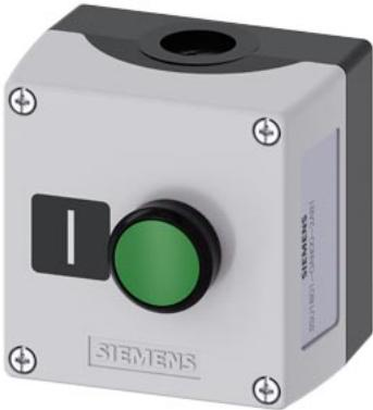
Enclosure for command devices, 22 mm, round, Enclosure material plastic, enclosure top part gray, 1 control point plastic, Recess for label, A=Pushbutton green, label: I, 1 NO, screw terminal, floor mounting, Label enclosed
