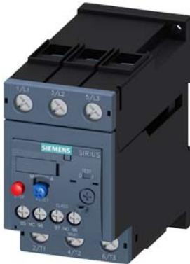
Overload relay 54...65 A Thermal For motor protection Size S2, Class 10 Stand-alone installation Main circuit: Screw Auxiliary circuit: Screw Manual-Automatic-Reset
