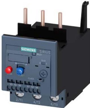
Overload relay 36...45 A Thermal For motor protection Size S2, Class 10 Contactor mounting Main circuit: Screw Auxiliary circuit: spring-type terminal Manual-Automatic-Reset
