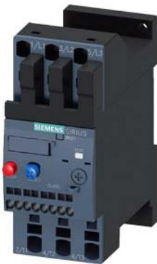
Overload relay 30...36 A Thermal For motor protection Size S0, Class 10 Stand-alone installation Main circuit: Spring-type terminal Auxiliary circuit: spring-type terminal Manual-Automatic-Reset
