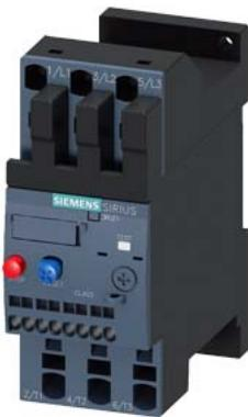
Overload relay 14...20 A Thermal For motor protection Size S0, Class 10 Stand-alone installation Main circuit: Spring-type terminal Auxiliary circuit: spring-type terminal Manual-Automatic-Reset
