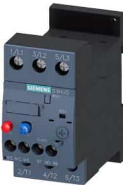
Overload relay 14...20 A Thermal For motor protection Size S0, Class 10 Stand-alone installation Main circuit: Screw Auxiliary circuit: Screw Manual-Automatic-Reset
