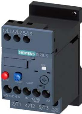
Overload relay 5.5...8.0 A Thermal For motor protection Size S00, Class 10 Stand-alone installation Main circuit: Screw Auxiliary circuit: Screw Manual-Automatic-Reset
