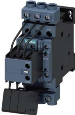
capacitor contactor, AC-6b 33 kVAr, / 400 V, 3-pole, 110 V AC, 50 Hz / 120 V, 60 Hz, auxiliary contacts: 1 NO + 2 NC, screw terminal, size: S0
