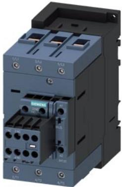
power contactor, AC-3e/AC-3, 110 A, 55 kW / 400 V, 3-pole, 230 V AC, 50 Hz, auxiliary contacts: 2 NO + 2 NC, screw terminal, size: S3, removable auxiliary switch
