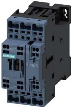
power contactor, AC-3e/AC-3, 32 A, 15 kW / 400 V, 3-pole, 21-28 V AC/DC, 50/60 Hz, with integrated varistor, auxiliary contacts: 1 NO + 1 NC, spring-loaded terminal, size: S0
