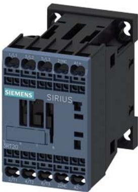
power contactor, AC-3e/AC-3, 9 A, 4 kW / 400 V, 3-pole, 24 V DC, auxiliary contacts: 1 NC, spring-loaded terminal, size: S00
