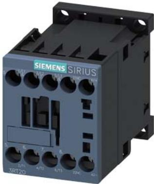
power contactor, AC-3e/AC-3, 9 A, 4 kW / 400 V, 3-pole, 24 V DC, 0.7-1.25\* Uc, with integrated diode, auxiliary contacts: 1 NC, screw terminal, frame size: S00, suitable for PLC outputs, no auxiliary switch can be added
