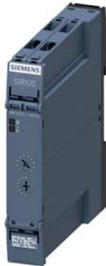
Timing relay, OFF delay with control signal 1 change-over contact, 15 time ranges 0.05 s...100 h 12-240 V DC, Wide voltage range at 50/60 Hz AC with LED, Screw terminal
