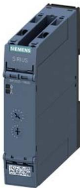
Timing relay, electronic on-delay 2 change-over contacts, 7 time ranges 0.05 s...100 h 24 V AC/DC at 50/60 Hz AC with LED, screw terminal
