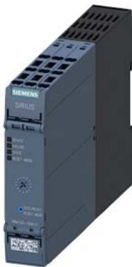
reversing starter, 3RM1, 500 V, 0 - 0.12 kW, 0.1 - 0.5 A, 110-230 V AC, screw/spring-loaded terminals (push-in)
