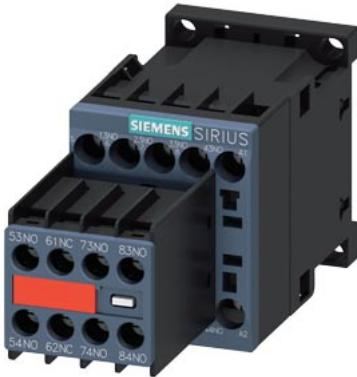
contactor relay, 7 NO + 1 NC, 110 V AC, 50 Hz / 120 V, 60 Hz, screw terminal, frame size S00, captive auxiliary switch
