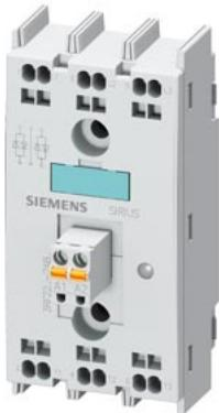
semiconductor relay, 3-phase 3RF2 55 A / 40 °C 48-600 V / 4-30 V DC 2-phase controlled spring-loaded terminal blocking voltage 1200 V for mounting on available cooling surfaces
