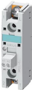
semiconductor relay, 1-phase 3RF2 width 22.5 mm, 90 A 48-460 V / 110-230 V AC ring cable terminal for mounting on available cooling surfaces
