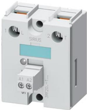
semiconductor relay, 1-phase 3RF2 width 45 mm, 30 A 48-460 V / 24 V DC screw terminal instantaneous switching for mounting on available cooling surfaces
