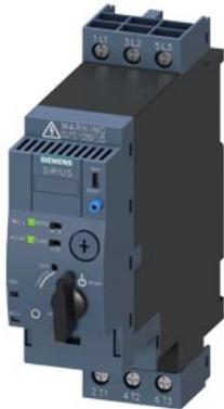
SIRIUS Compact load feeder DOL starter 690 V 24 V AC/DC 50...60 Hz 0.32...1.25 A IP20 Connection main circuit: screw terminal Connection auxiliary circuit: plug-in, without terminals
