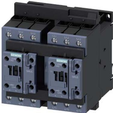
reversing contactor assembly, AC-3e/AC-3, 51 A, 22 kW / 400 V, 3-pole, 110 V AC, 50 Hz / 120 V, 60 Hz, screw terminal, electrical and mechanical interlock, auxiliary contacts: 2 x 1 NO
