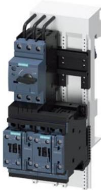
Load feeder fuseless, Reversing duty 400 V AC, Size S0 4.50...6.30 A 24 V DC screw terminal for 60 mm busbar systems (also fulfills type of coordination 1) Type of coordination 2,  $I_q = 150$  kA 1 NO+1 NC (contactor)
