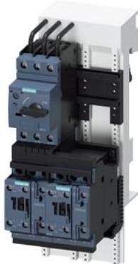
Fuseless motor starter Reversing operation 600VAC Size S0 1.4-2A 220/240VAC 50/60HZ screw connection For snapping onto 60 mm busbar systems Type of coordination 2 IQ = 150 KA Also full fills type Of coordination 1 1NO+1NC (per contactor)
