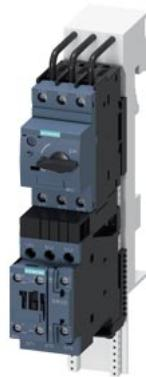
Fuseless motor starter Direct start 600VAC Size S0 1.8-2.5A 24V DC screw connection For snapping onto 60 mm busbar systems Type of coordination 2 IQ = 150 KA Also full fills type Of coordination 1 1NO+1NC (contactor)
