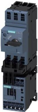
Load feeder fuseless, Direct-on-line starting 400 V AC, Size S00 7.00...10.0 A 230 V AC Spring-type terminal for installation on standard mounting rail Type of coordination 1,  $I_q = 150$  kA 1 NO (contactor)
