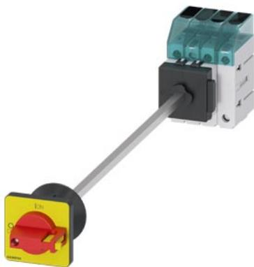
Load disconnector 3LD3, Iu 32 A Main switch 3-pole + N Rated operating capacity for AC-23 A at 400V 11.5kW floor mounting Basic switch with door coupling Central hole mounting 22.5mm Toggle drive red / yellow 48x48 mm
