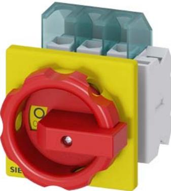
SENTRON, Switch disconnector 3LD, emergency switching-off switch, 3- pole, Iu: 25 A, operating power / at AC-23 A 400 V: 9.5 kW, front-mounted, 1 NC, 1 NO, rotary operating mechanism, Red / yellow, 4-hole mounting of the handle
