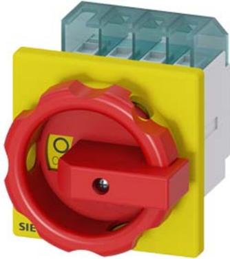
SENTRON, Switch disconnecter 3LD, emergency switching-off switch, 4- pole, Iu: 16 A, operating power / at AC-23 A 400 V: 7.5 kW, front-mounted, rotary operating mechanism, Red / yellow, 4-hole mounting of the handle
