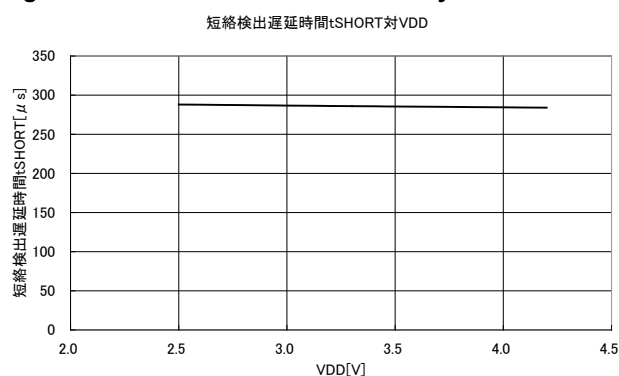
Figure 11. Short-circuit Detection Delay Time vs. VDD
