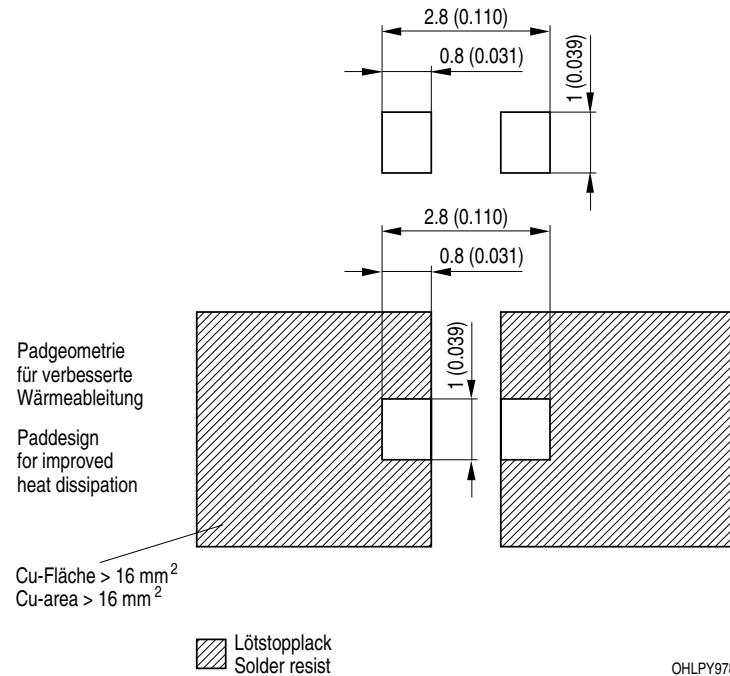
For superior solder joint connectivity results we recommend soldering under standard nitrogen atmosphere.
