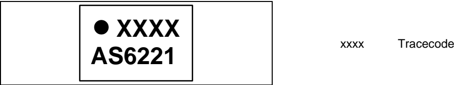
Figure 16: WLCSP package marking/code for AS6221
