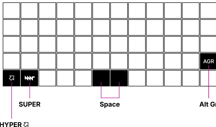
Pocket Reform has a mechanical “ortholinear”<sup>1</sup> keyboard with 60 keys.
