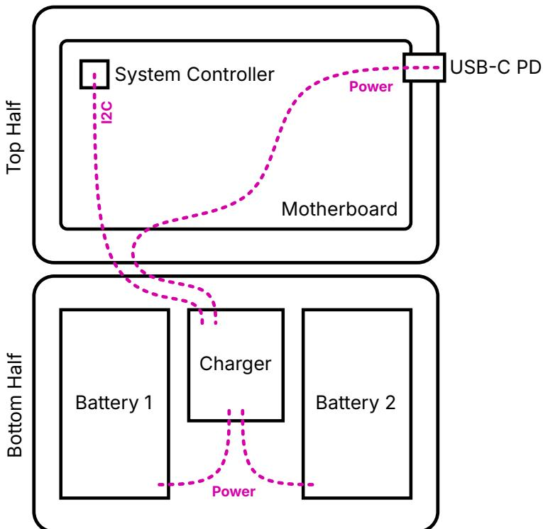
Underneath the keyboard reside two LiPo battery cells with 606090 form factor. In their middle: the charger board. This little PCB mainly contains two chips: one is a fuel gauge with battery protection (MAX17320G20+), and one is the actual charger, the MPS MP2650. These chips are decoupled from the motherboard to allow for future flexibility in terms of battery architectures and chemistries, and to allow both the motherboard and the charger to be reused in other contexts.
