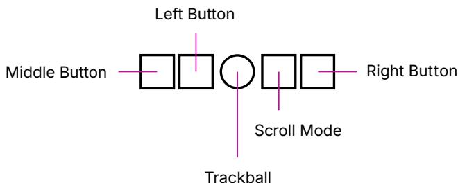
The trackball works like a mouse with four buttons: middle button, left click, scroll button, and right click. Roll the ball to move the cursor. Pressing the *Middle Button* and the *Scroll Mode* button simultaneously activates *Sticky Scroll Mode*, so
