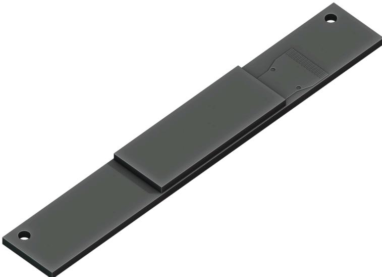
The OLED display sits on the OLED Module which is connected to the keyboard through a 4-pin, 1 mm pitch flex cable. The communication protocol is I<sup>2</sup>C. The module is mounted in the Main Box on top of the keyboard with two M2×4 pan head screws.
