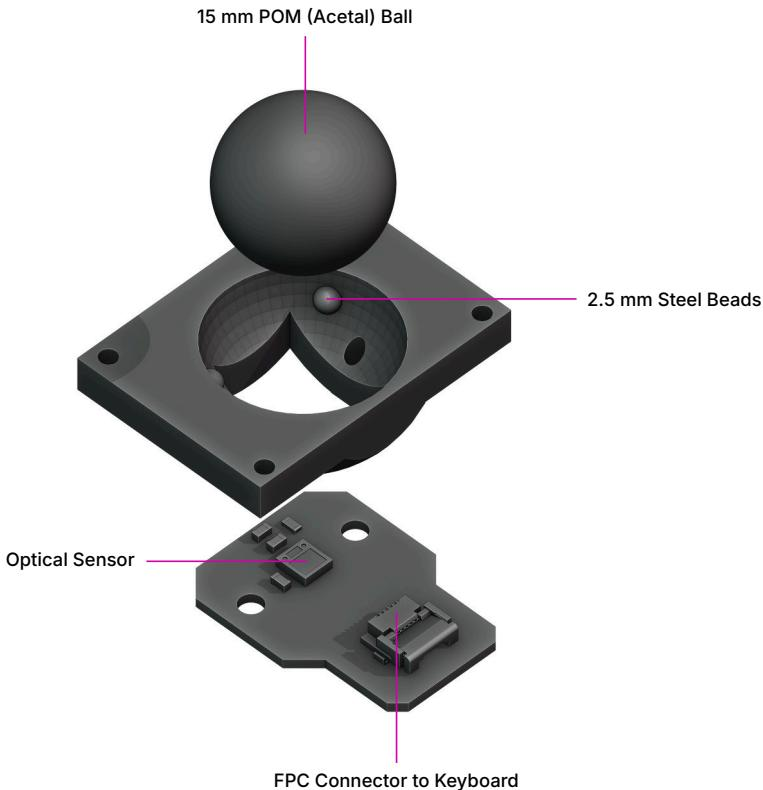
The trackball uses an RP2040 microcontroller to convert X and Y movement coordinates from the PAT9125EL optical sensor that is connected via I<sup>2</sup>C to the USB HID Mouse protocol. The electronic connection between trackball sensor and controller is made with a 6-pin 0.5mm pitch flex cable.
