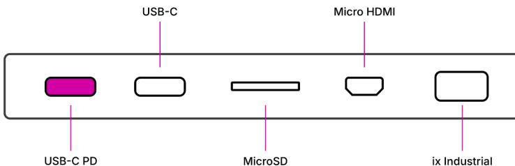
The Right Port Cover is also attached with 2 M2 screws and exposes the 5 ports of the motherboard:
