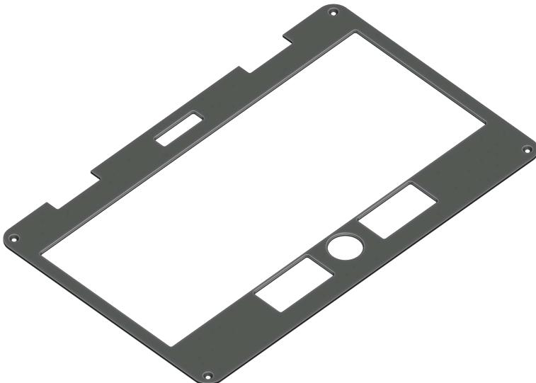
The keyboard frame is a 1.2 mm thick anodized milled aluminum plate that acts as the bezel for the keyboard, trackball, and the OLED display. It is attached with 4 M2 screws.
