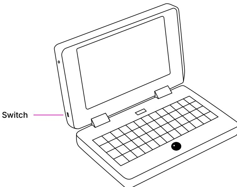
Move the switch away from the hinges to turn the standby power on. Move the switch towards the hinges to turn it off.
