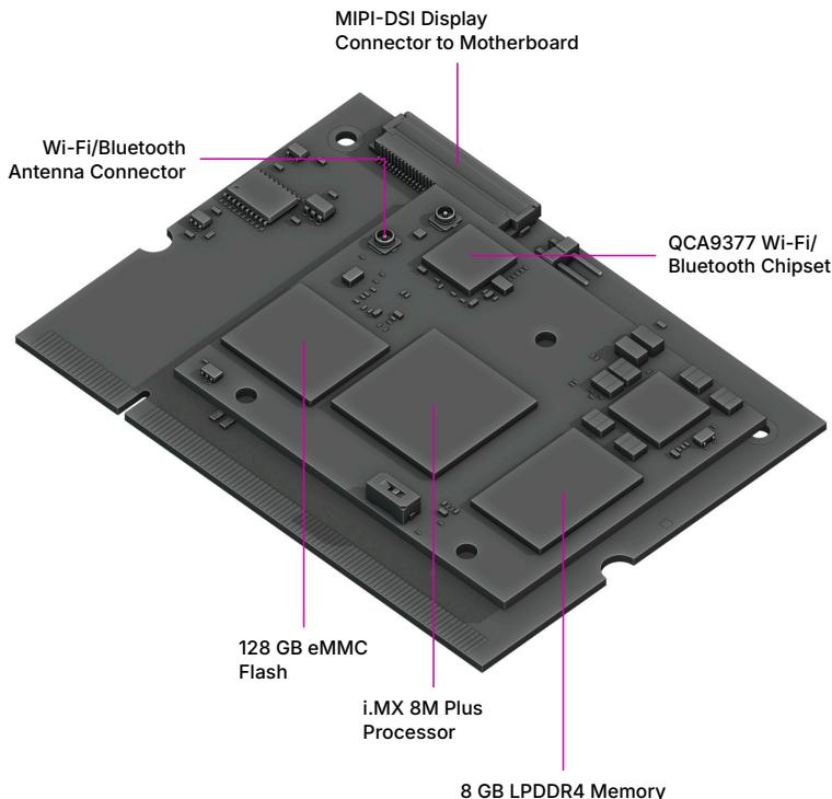
The first version of the MNT Pocket Reform ships with an NXP i.MX8M Plus Processor Module. We are constantly developing new modules for Pocket Reform with different
