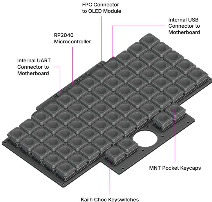
The keyboard is mounted to the top of the Bottom Half with six M2×4 pan head screws. It is powered by an RP2040 32-bit microcontroller. The controller scans the row/column matrix of keyswitches and reports key presses via USB HID (human interface device) to the motherboard. Each switch has a diode to prevent ghosting, so you can press multiple keys at once. The microcontroller runs a firmware based on TinyUSB, which is an open source library for implementing USB devices.
