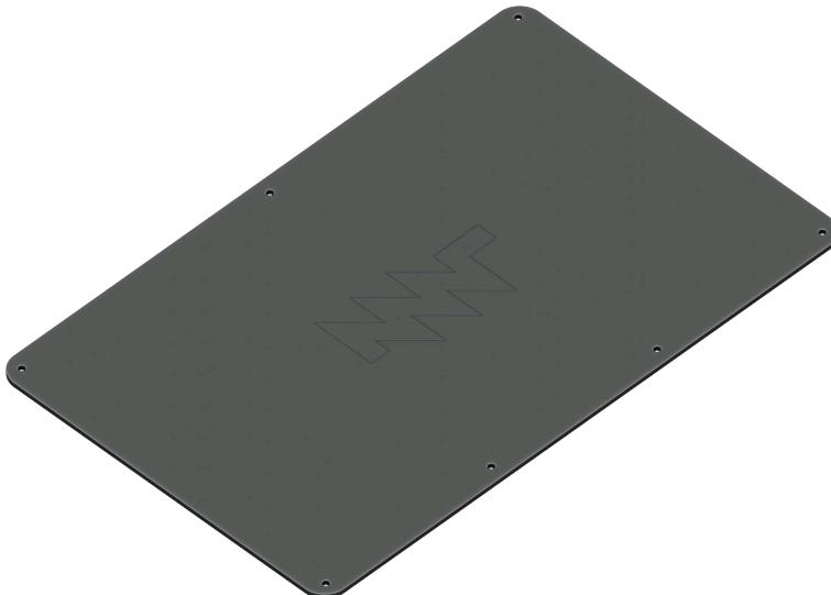
The top back cover is a 1.2 mm PCB that covers the motherboard. There is a large exposed copper area in the middle of the cover. It serves as the heatsink and has to be thermally attached to the CPU processor module using a square of a 2 mm thick thermal pad. It is attached with 7 M2 screws.
