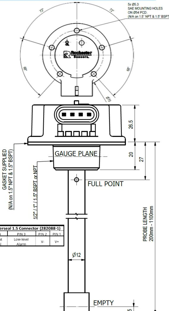
Standard part numbers and options. Contact Rochester Sensors for other length and output
