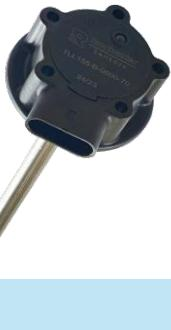
The TLL155 liquid level sensor is designed for use in fuel tanks and is available with a variable resistive, voltage or current output suitable for driving industry standard fuel gauges or connecting into PLCs. It is supplied in standard probe lengths of 500mm or 1000mm and can be cut to suit the length required at site. For volume production requirements we will manufacture to the length & output you require.
